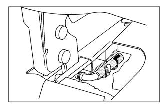
The driver's side pin has a gray cap with a black "L" marked on it.
